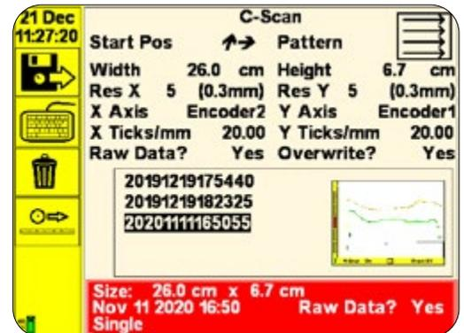
Scanner Control Menu facilitates rapid setup of an automated scan.
