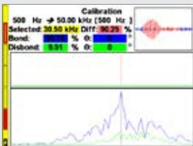
Pitch-Catch Mode calibration showing the bond and dis-bond spectrum.
