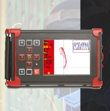
Designed to meet & exceed the requirements of EN 1711 & ISO 17643 "Eddy Current Examination of Welds by Complex Phase Analysis".
