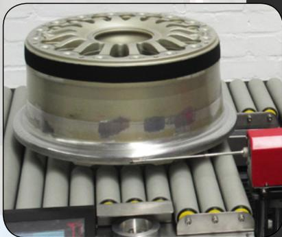
Flexible set up with automatic wheel adaptation and direction of test.
