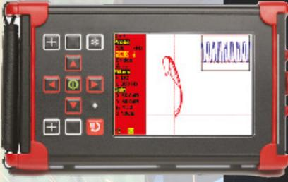
Designed to meet & exceed the requirements of EN 1711 & ISO 17643 "Eddy Current Examination of Welds by Complex Phase Analysis".
