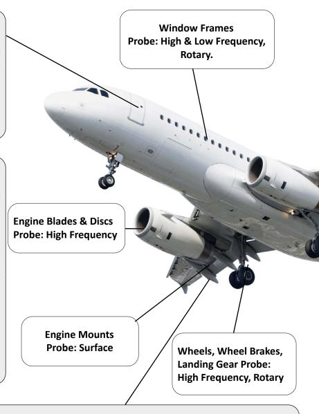
Area of Inspection: Wing & Surface Hinges Probe: High & Low Frequency
