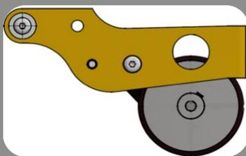
A rotary encoder to provide distance information to the software and synchronise the sample rate with the speed.
