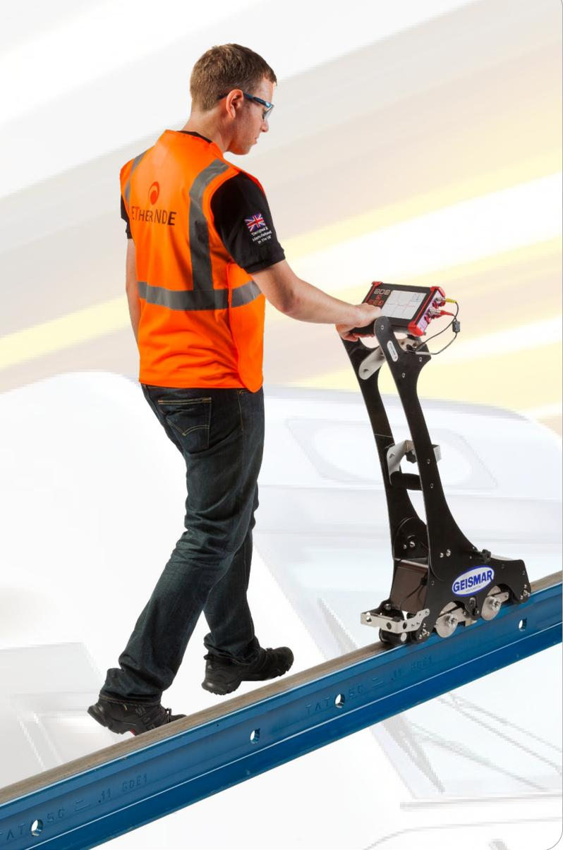
The FILUS EC-1 Trolley is a hand-pushed trolley, specially designed to check a single rail using Eddy current methods.
