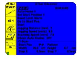
• The PhaseCheck C-Scan menu allows easy, flexible encoder setup and scan parameter setting. Can be used with a single axis encoder to produce a C-Scan.
