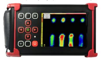
They say "A picture is worth a 1000 words", to date "pictures" (C-Scans) in eddy current have been limited to expensive large laboratory instruments. Now for the first time C-Scan data is available in a hand-held eddy current flaw detector package, the PhaseCheck.
