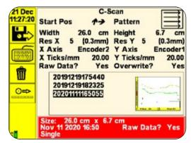
Scanner Control Menu facilitates rapid setup of an automated scan.
