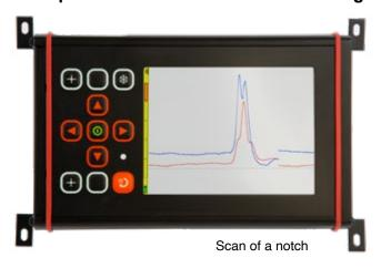
The AMCheck can be conveniently panel mounted for inspection of Additive Manufactured (AM) parts during inspection.
