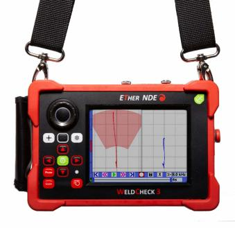
With its improved mechanical and ergonomic design the WeldCheck3 brings ETher NDE's WeldCheck series right up to date. Based on in-field inspection feedback and embracing the use of new materials, the WeldCheck 3 delivers to the end-user enhanced ruggedness, a toughened screen, improved connector access and performance, combined with optional features such as an encoder wheel.
