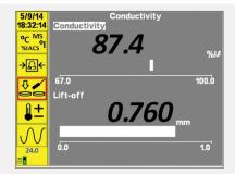
CONDUCTIVITY MEASUREMENT: Many of the Aerospace procedures require that Conductivity Measurement is available on the designated Eddy Current Flaw Detector.
