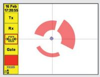
Impedance Plane (XY) Trace with multiple sector gates
