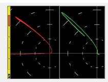
AUTO-MIX FEATURE: A dual frequency mix exploits the phase and sensitivity change between two different types of indication to suppress one and enhance the other.
