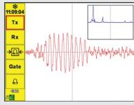
RF (A-Scan Waveform) with Frequency Spectrum Inset
