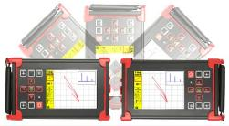
The ETHERCHECK has the ability to be used in left and right-handed mode; thanks to the "Auto Flip" function. This is especially useful if the operator is inspecting in a restricted area like the Engine Mounts.
