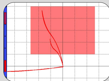
XY Full Screen with Box Alarm
